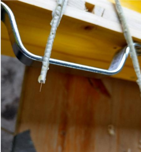
**Fig. 13** Ruptured casted cable solution.
