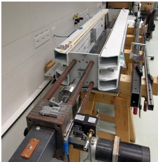
Fig. 18 Pull-out box and its step motor.
