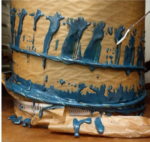
**Fig. 32** Effects of temperature exposition on the tight section of M4.
