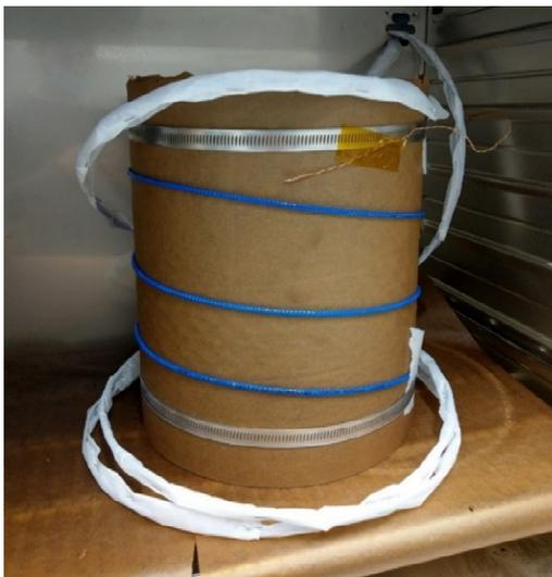
*Fig. 15 Cable setup in the oven.*
