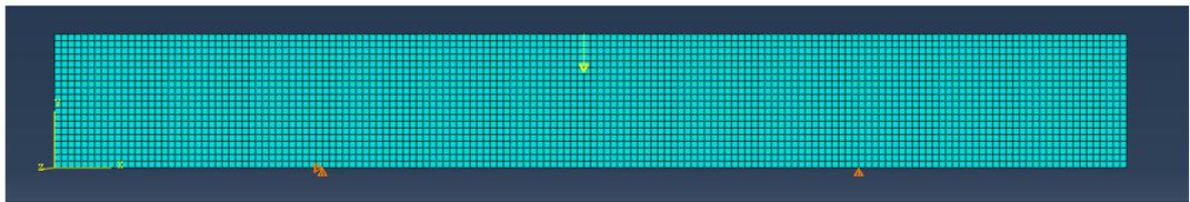
**Fig. 55** Finite element model of the bending test.
