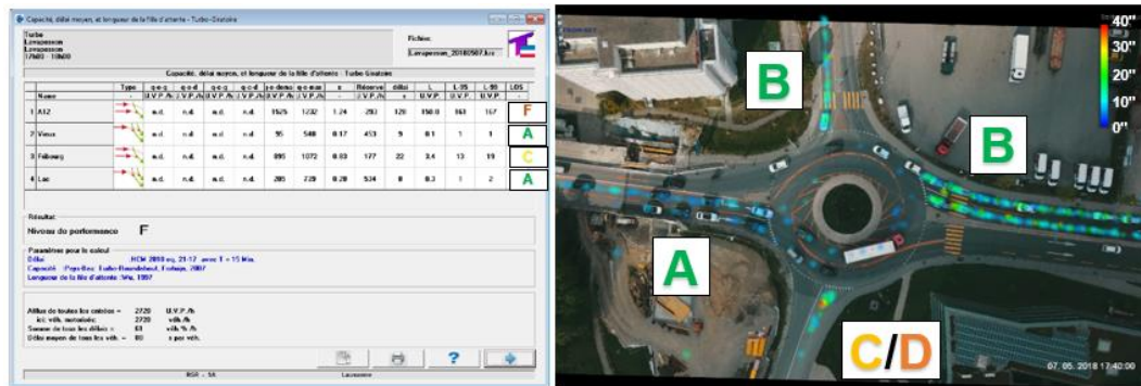
Fig. 110 Lavapesson – Niveau de service – Turbo-Roundabout, Fortuijn, 2007.
