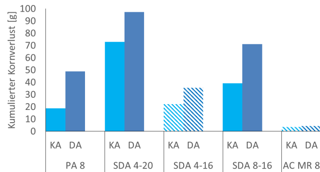
Fig.15 Aggregate loss after 10 double cycles for asphalt mixtures SDA 4-20, SDA 8-16 and PA 8 as well as SDA 4-16 and AC MR 8 (hatched) in comparison between Karlsruhe and Darmstadt (Figure 15 in main document)
