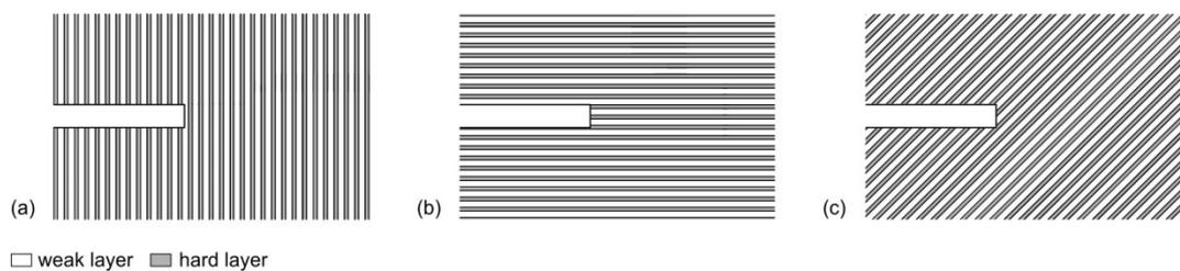
**Figure 1.2.** Investigated orientations of the layers to the tunnel axis for a sequence of alternating weak and hard rocks.
