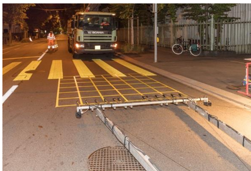
Fig. 80 Installed ETH Delta device before the test above sensor section 1 of the grid
