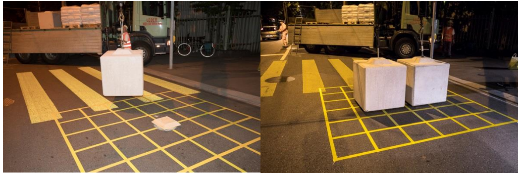
Fig. 83 Positioning of the concrete block on a wooden bearing on top of a sand cushion during test series S4 (test K1) Fig. 84 Position of two concrete blocks during test series S4 (test K2)
