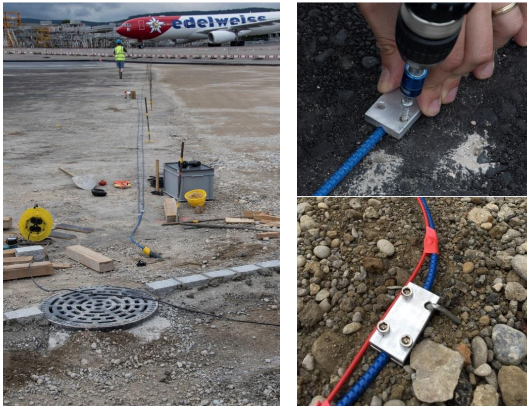
Fig. 42 Prestressing of sensors (left); fixation of cable clamps using screws (top right); fixation of sensing cable using a pair of clamps and a peg (bottom right) at Zurich Airport test site
