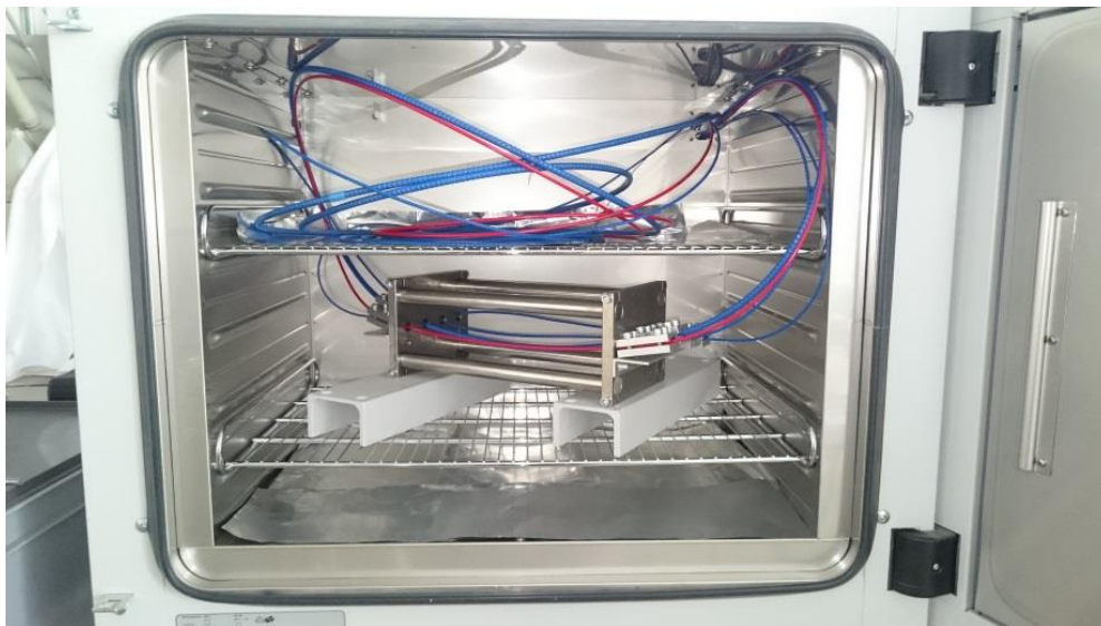
Fig. 19: Setup for testing the thermal behavior of the sensing cables
