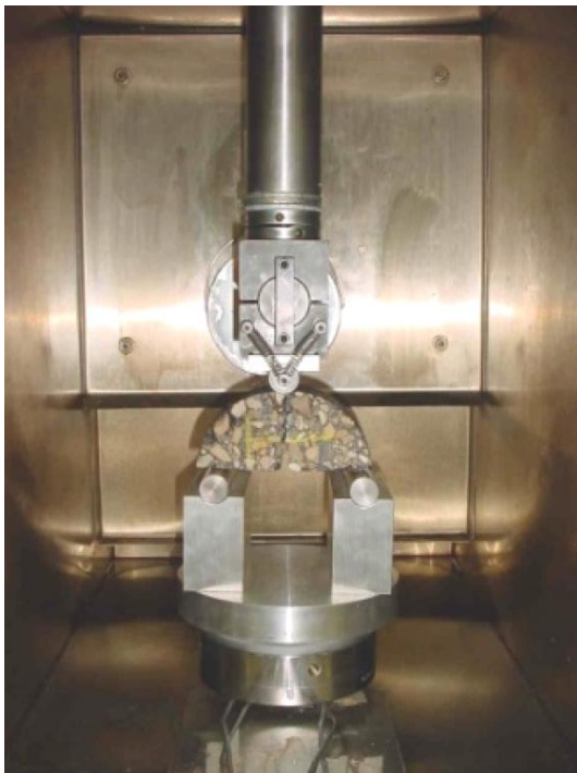
Abb. 12 Halbkreis-Biegetest (Semi-Circular Bending Test; Mohammad et al., 2012 [44]).
