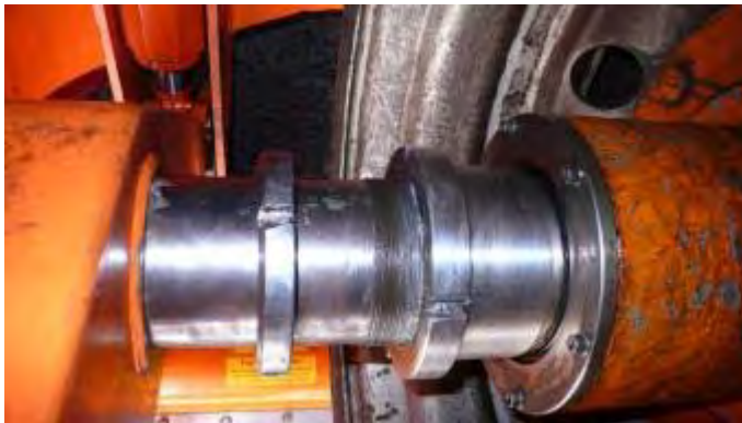
Fig. 5.22 Picture showing the insecure fixation of the trafficking wheel
