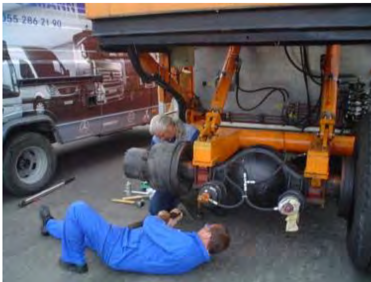
Fig. 7.5 Revision of the machine breaks.
