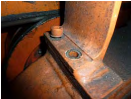
Fig. 6.7 Failure of a bolt in a C-Bracket
