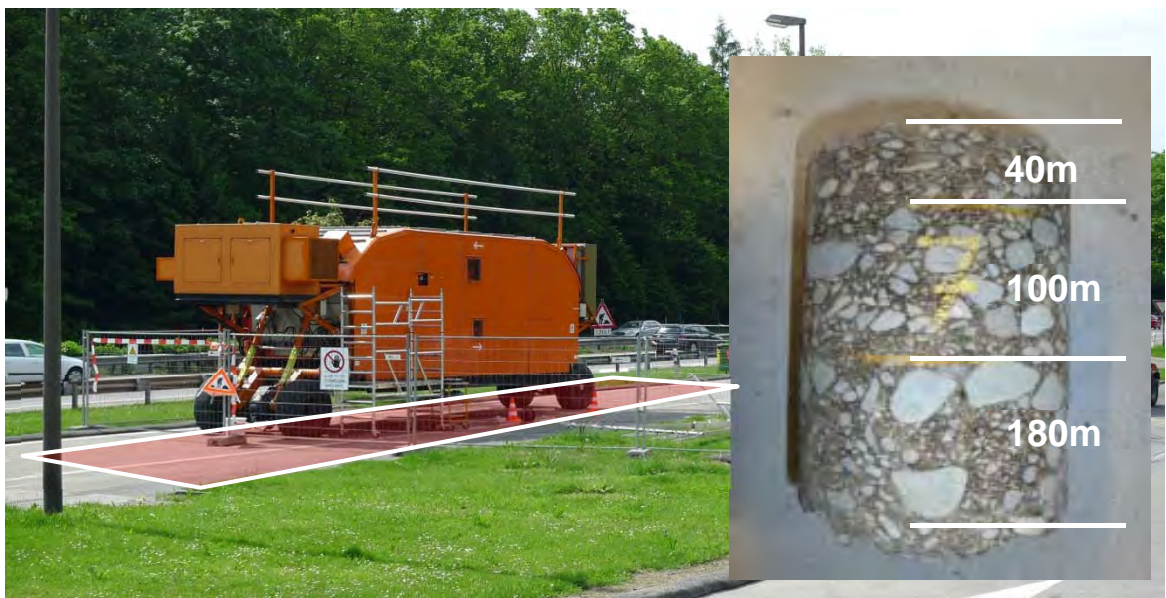
Fig. 6.3 View of testing site and thickness of the pavement
