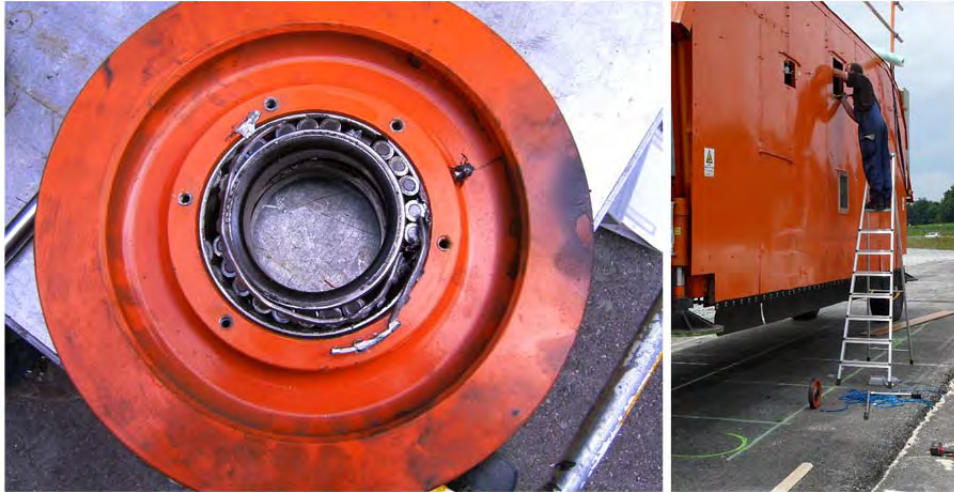
Fig. 5.21 Damaged bearing (left) and replacement work carried out in Filderren (right).
