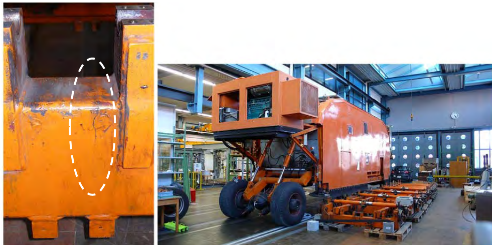
Fig. 5.20 Crack in the old bogies (left) and replacement work carried out at Empa (right)
