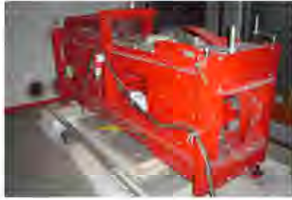
Figure 10. MMLS3 trafficking of extracted slab.
