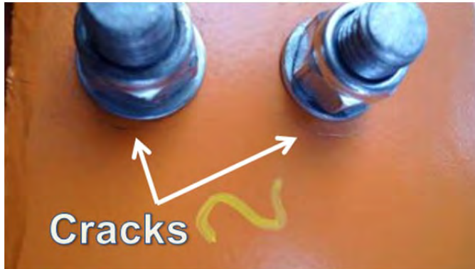
Fig. 7.6 Crack in a bolt fixation area
