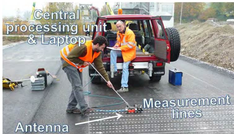
Fig. 5.9 Inspection of the pavement with GPR.
