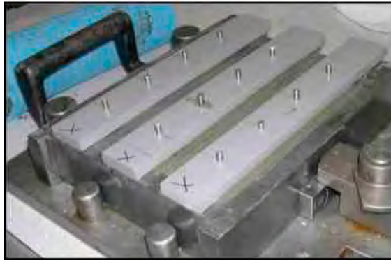
Figure 11: Samples of grout mixture for measuring the evolution of the electrical resistance with time. a) moulds after filling with grout on the vibration table.
